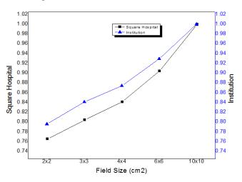
Fig. 7. Un-calibrated Output Factor Dataset for 6 MV X-Ray.
