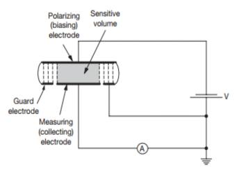
**Fig. 4.** Circuitry of a dosimetry system which is based on ionization chamber [12]
