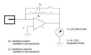
**Fig. 6.** Electrometer in Feedback Mode of Operation[12]
