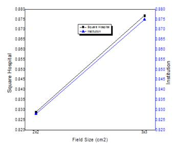
Fig. 10. Calibrated Output Factor Dataset for 10 MV X-Ray.
