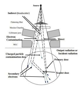
Fig. 2. Internal Construction of LINAC [11]
